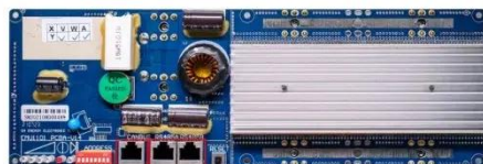
BS485 Communication between battery and inverters Band rate:9600bps BS485 Interface Communication between parallel packs of BMS and PC Band rate:9600bps
