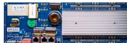
ES485 Communication between battery and inverter Band rate: 9600bps
